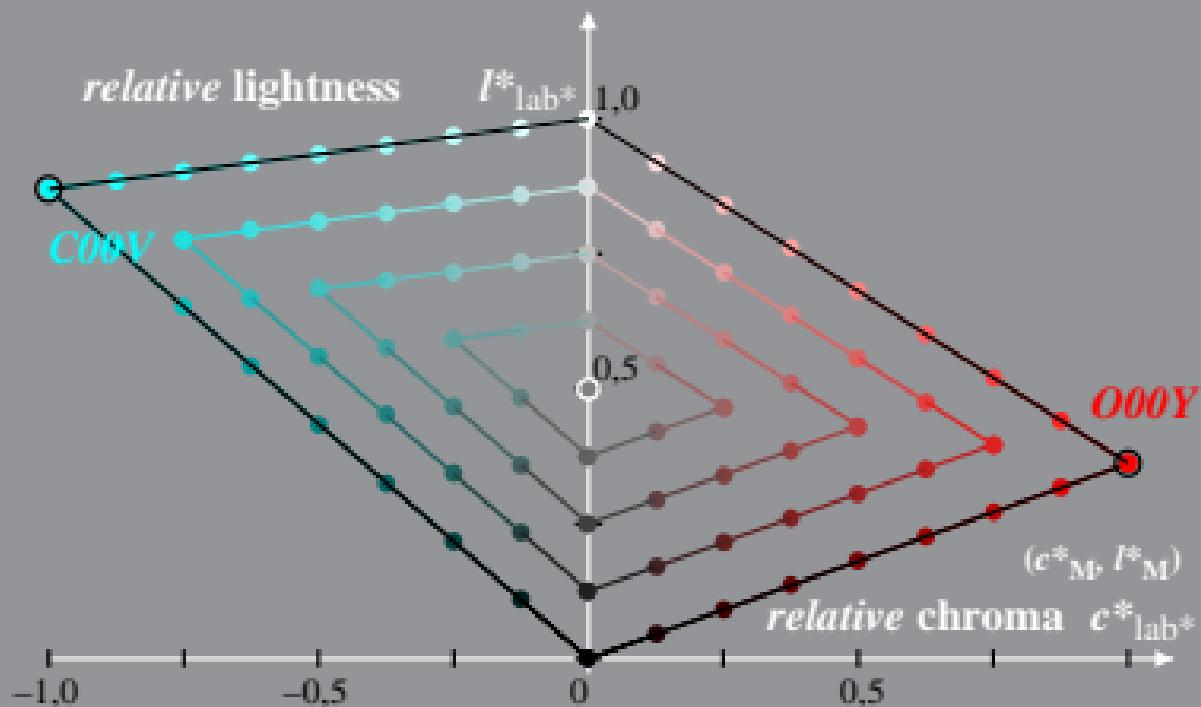
Adapted (a) CIELAB ( $C^*_{ab,a}$ ,  $L^*$ ) and relative CIELAB ( $c^*_{lab*}$ ,  $l^*_{lab*}$ )
