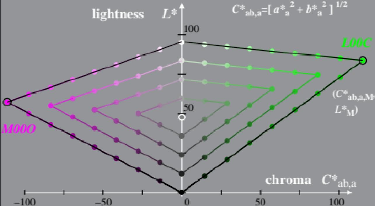
Linear relation CIELAB ( $L^*$ ,  $a^*$ ,  $b^*$ ) and adapted (a) CIELAB ( $C^*_{ab,a}$ ,  $L^*$ )
