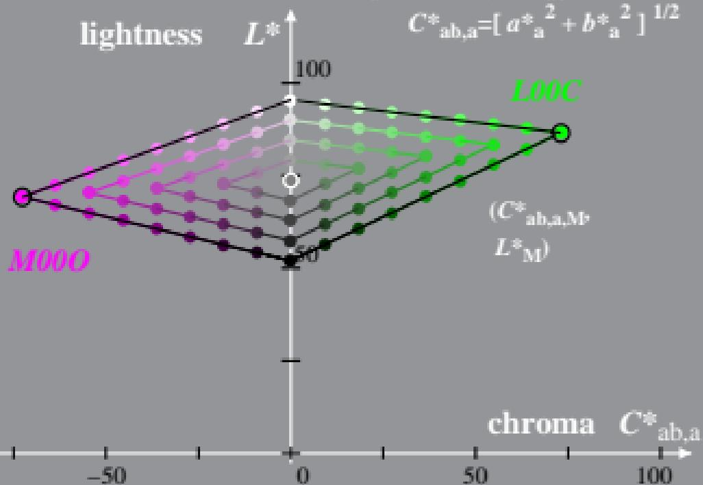
Linear relation CIELAB ( $L^*$ ,  $a^*$ ,  $b^*$ ) and adapted (a) CIELAB ( $C^*_{ab,a}$ ,  $L^*$ )
