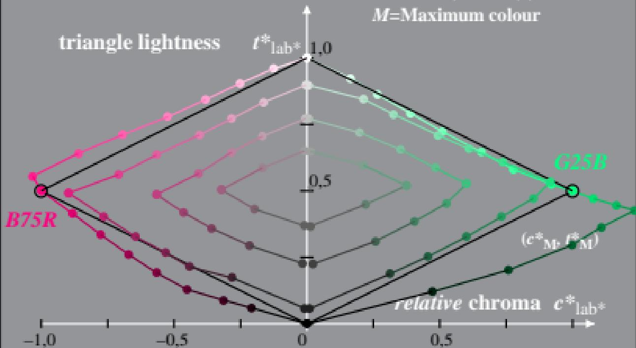
Linear relation adapted (a) CIELAB ( $C^*_{ab,a}$ ,  $L^*$ ) and relative CIELAB ( $c^*$ ,  $t^*$ )
