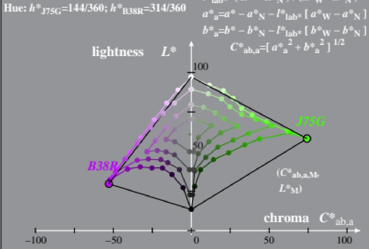
Linear relation CIELAB ( $L^*$ ,  $a^*$ ,  $b^*$ ) and adapted ( $a$ ) CIELAB ( $C^*_{ab,a}$ ,  $L^*$ )
