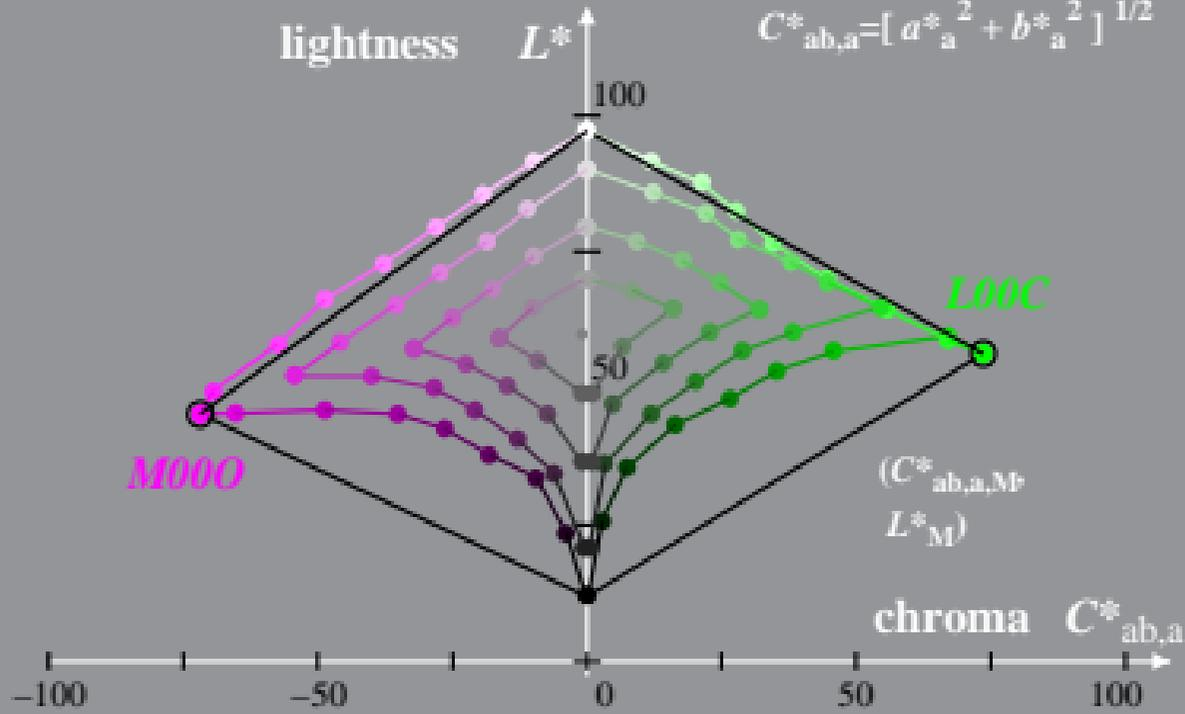
Linear relation CIELAB ( $L^*$ ,  $a^*$ ,  $b^*$ ) and adapted (a) CIELAB ( $C^*_{ab,a}$ ,  $L^*$ )
