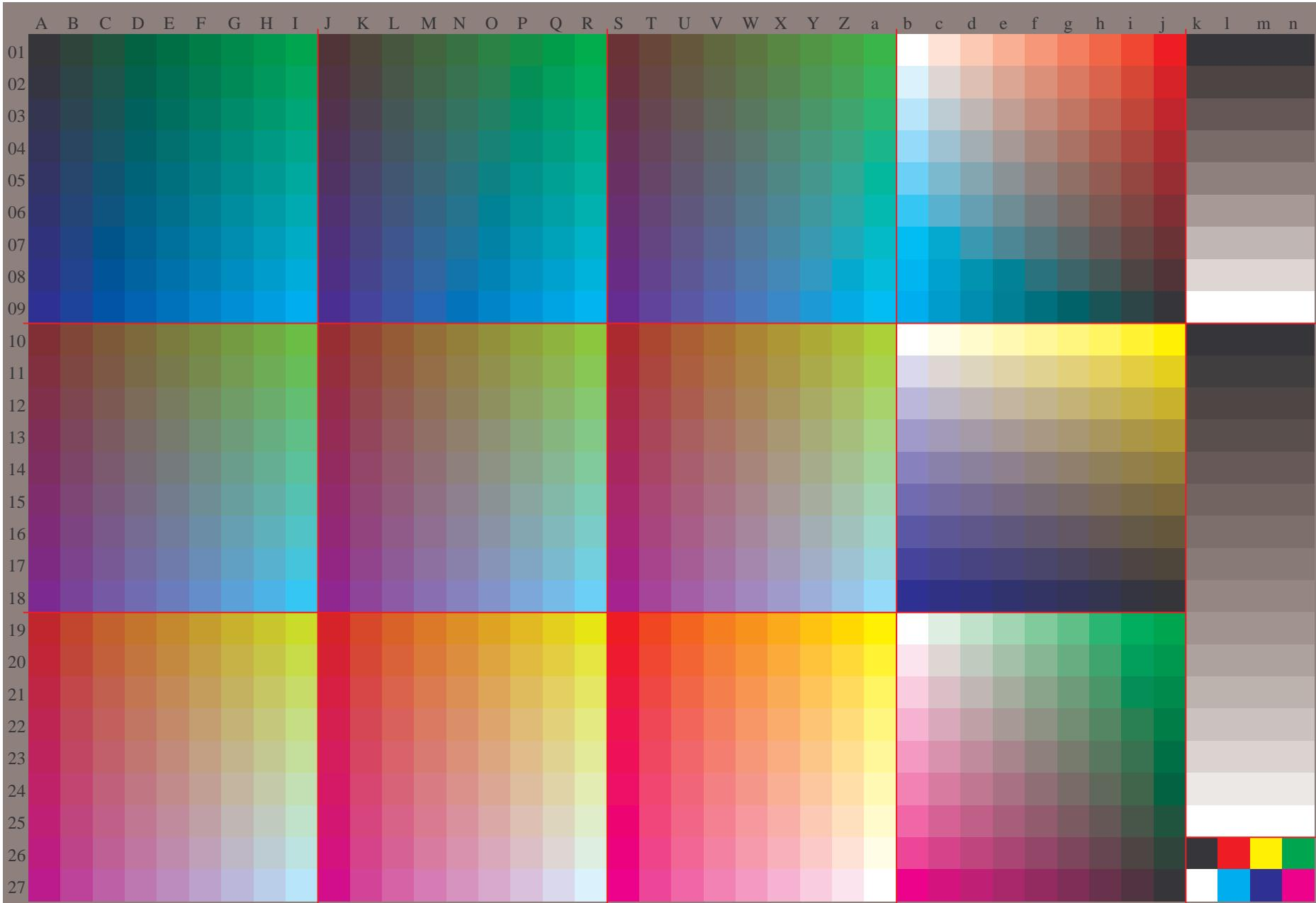
TUB-test chart GE61; Relative Device Colour System G
