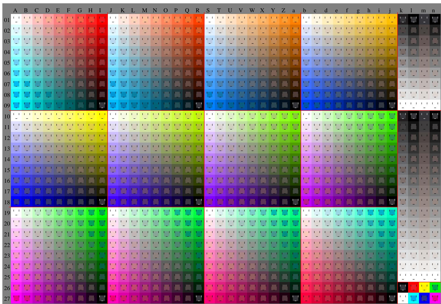
TUB-test chart GE46; Relative Device Colour System O
