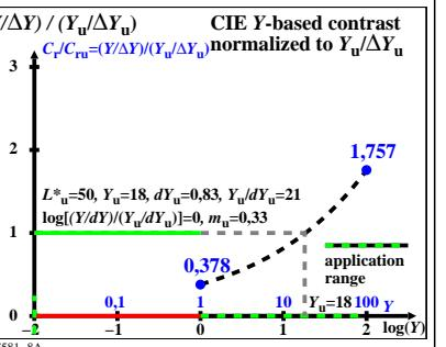
TUB-test chart EE58; Calculated for the CIELAB colour-difference formula, see ISO/CIE 11664-4
