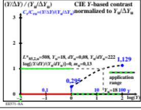
TUB-test chart EE57; Calculated for the LABJND colour-difference formula, see CIE 230:2019 lightness  $L^*$ , threshold  $\Delta Y$ , sensitivity  $\Delta Y / Y$ , contrast  $Y / \Delta Y$ , unnormalized and normalized
