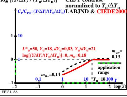
TUB-test chart EE33; Comparison of the LABJND and the CIEDE2000 colour-difference formula
