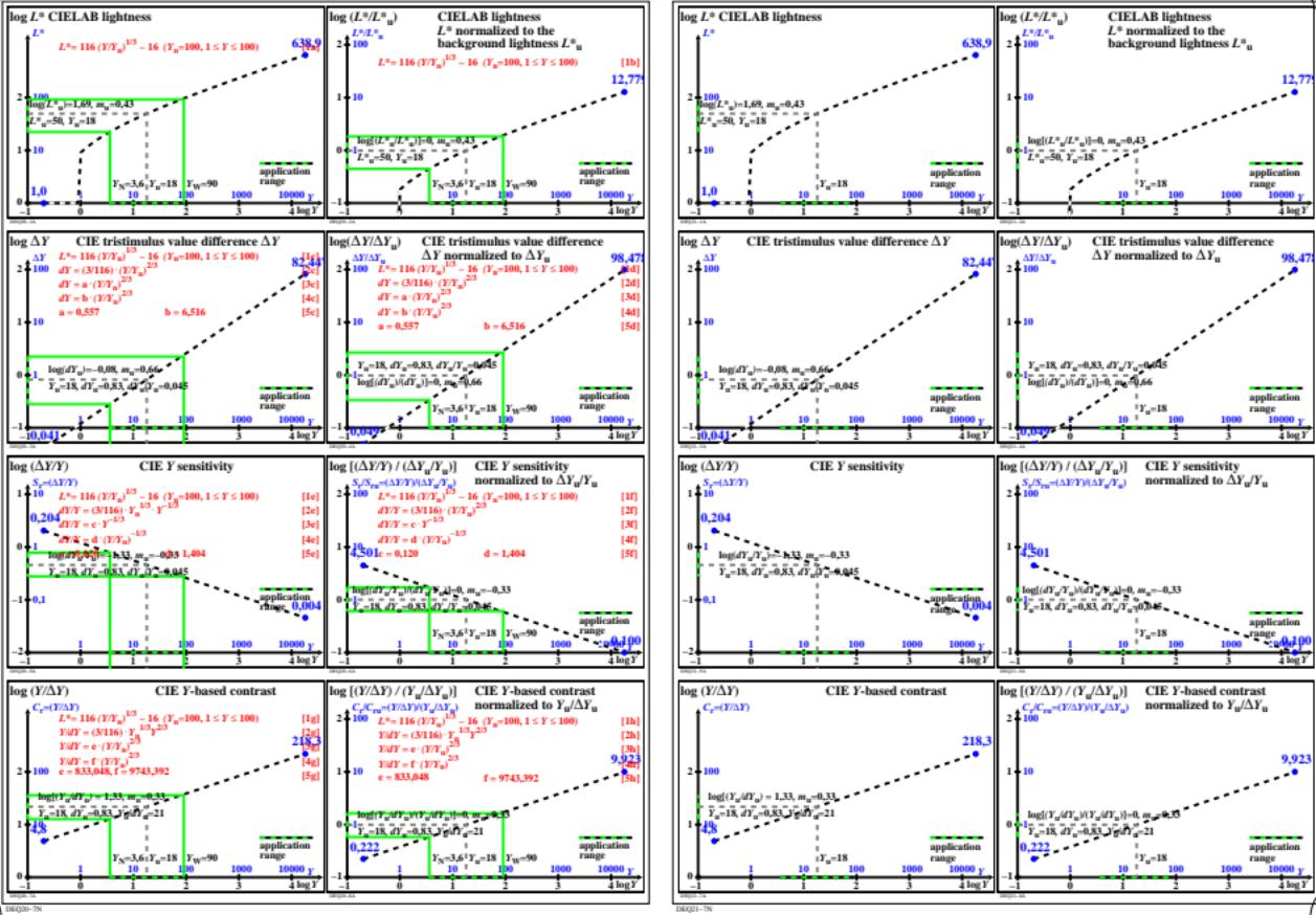
TUB-test chart DEQ2; For CIELAB colour-difference formula, see ISO/CIE 11664-4
