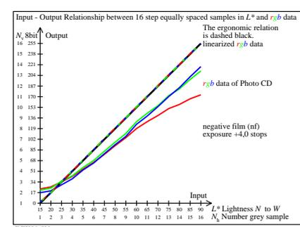
TUB-test chart DEK0; Input-Output relationship of  $L^*$ - $rgb$  data for slide (sf) and negative (nf) film
