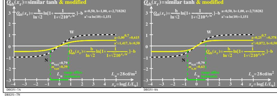
TUB-test chart DEG5; Model of response functions  $Q_{ab}(x_r)$  and deviations logarithmic response functions  $Q_{ab}(x_r)$  and deviations with  $e^{x_r/a}$  and  $10^{x_r/a}$ ;  $a^n=a^{0.7}$
