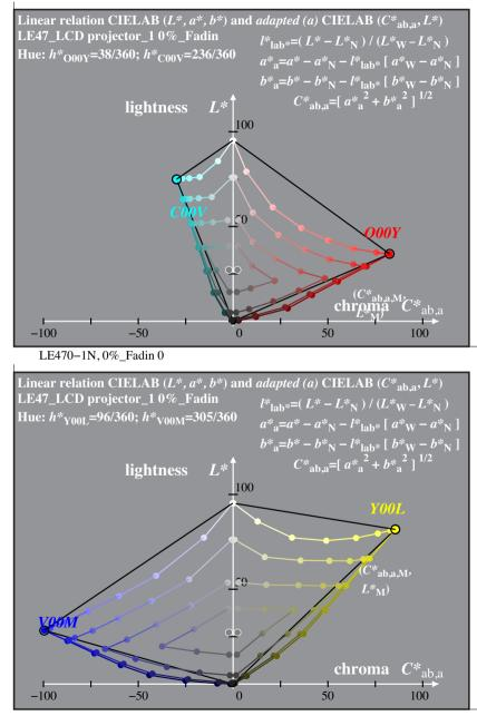
Fig. 2: CIELAB diagrams ( $C^*_{ab}$ ,  $L^*$ ) of sRGB display and LCD projector
