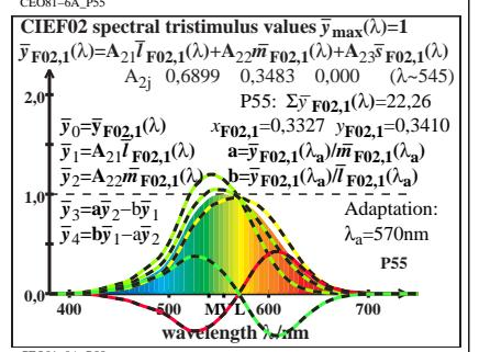
TUB-test chart CEO8; XYZ-CIEF\_02-degree colorimetry, CIE and R21 components of  $\bar{y}(\lambda)$
