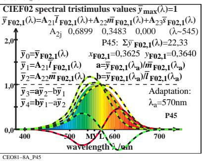
TUB-test chart CEO8; XYZ-CIEF\_02-degree colorimetry, CIE and R21 components of  $\bar{y}(\lambda)$
