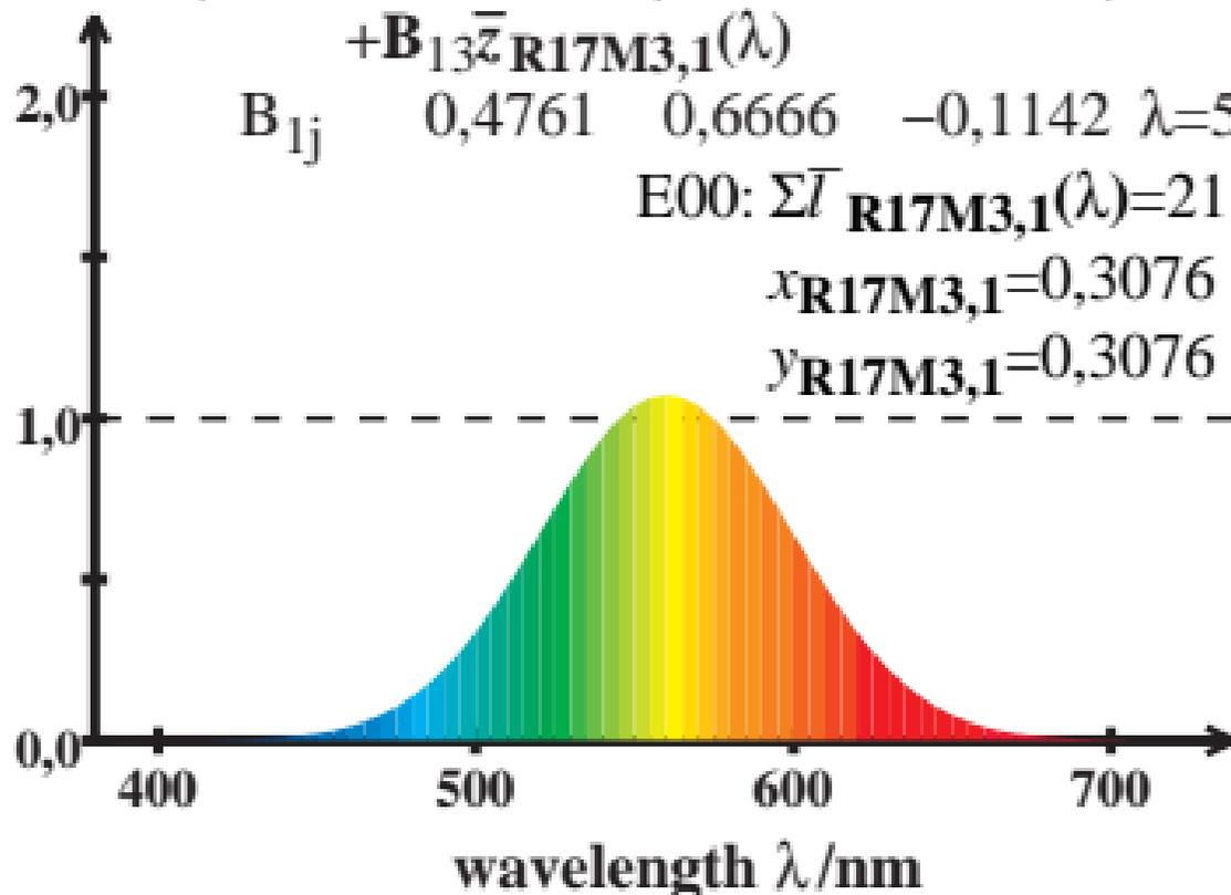
LMS\_R17M3 cone sensitivity  $\bar{y}_{\max}(\lambda)=1$
