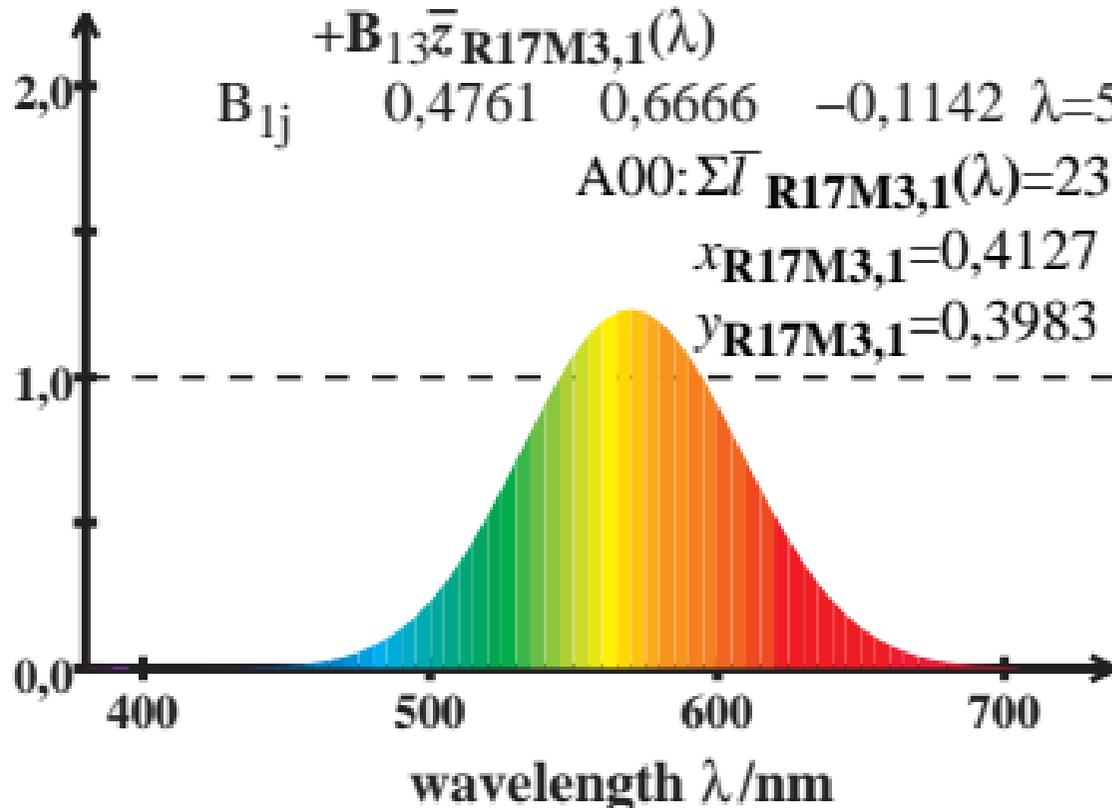
LMS\_R17M3 cone sensitivity  $\bar{y}_{\max}(\lambda)=1$
