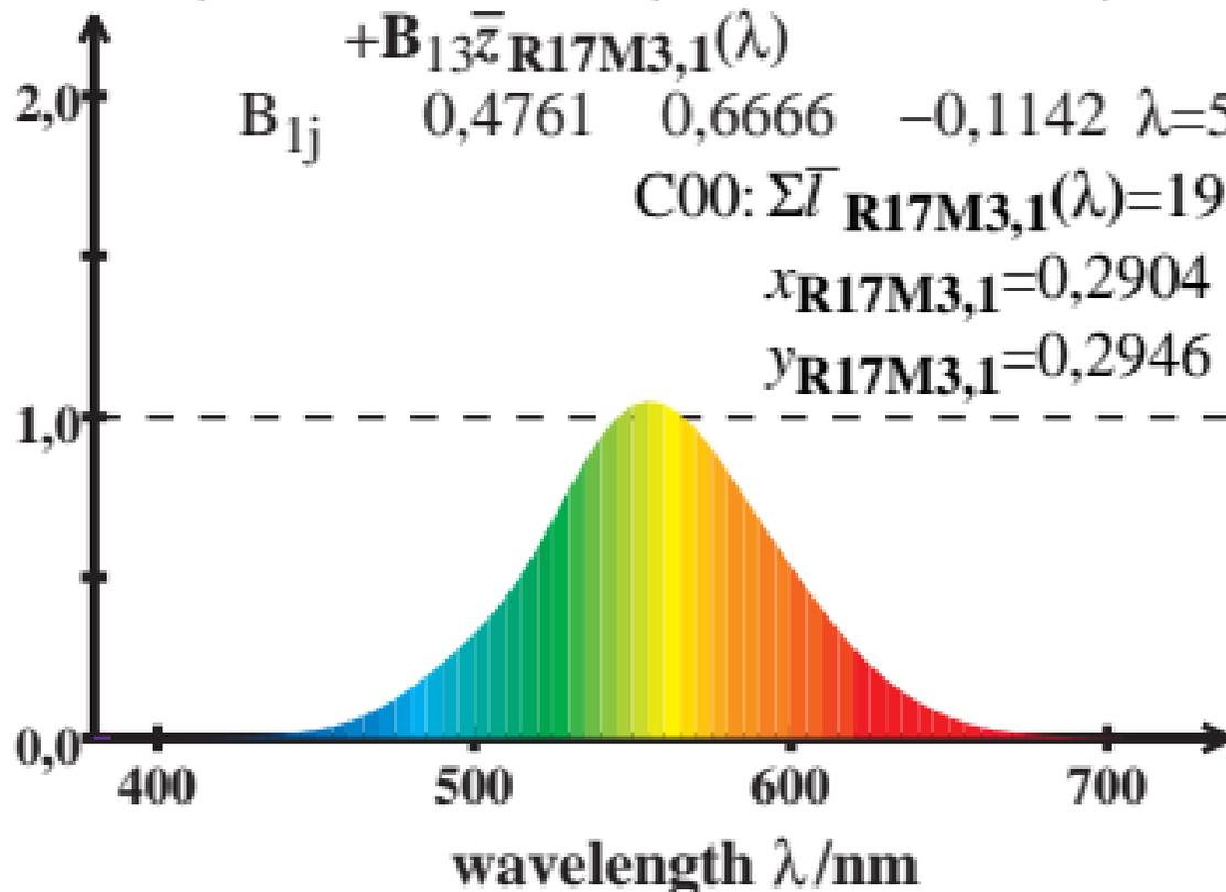
LMS\_R17M3 cone sensitivity  $\bar{y}_{\max}(\lambda)=1$
