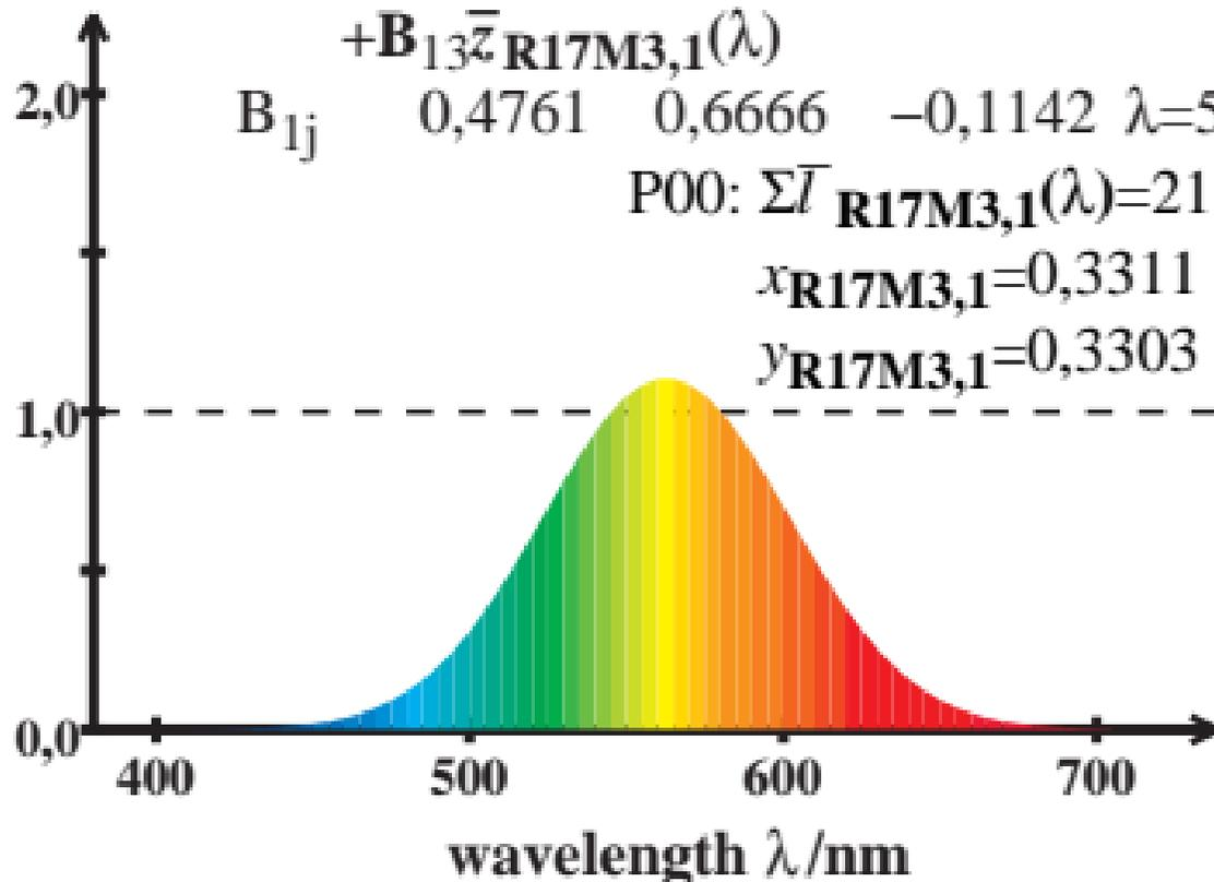
LMS\_R17M3 cone sensitivity  $\bar{y}_{\max}(\lambda)=1$
