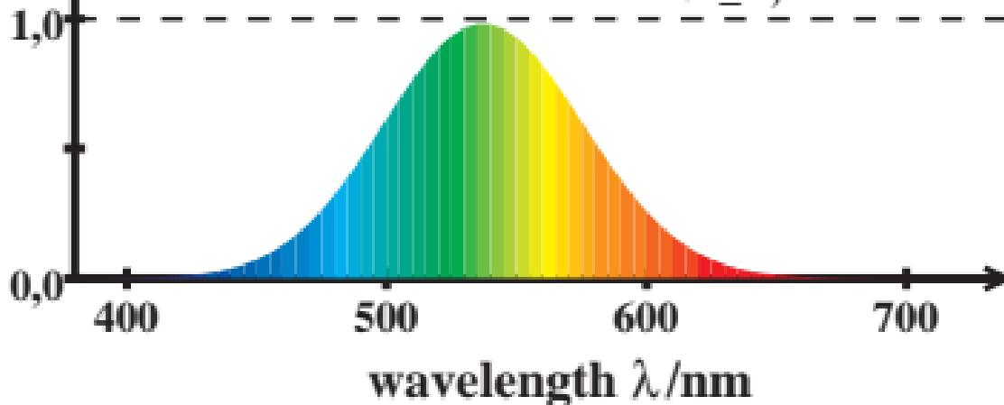
LMS\_F02\_L cone sensitivity  $\bar{y}_{\max}(\lambda)=1$
