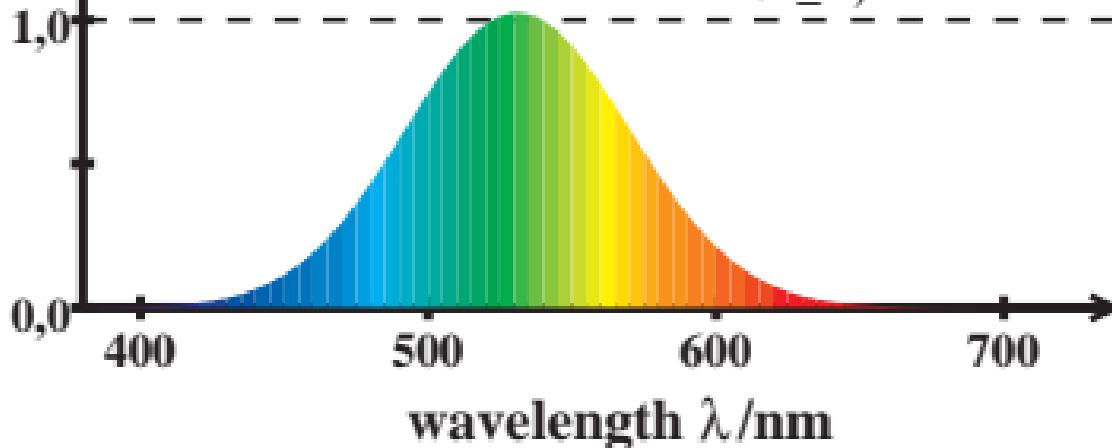
LMS\_F02\_L cone sensitivity  $\bar{y}_{\max}(\lambda)=1$
