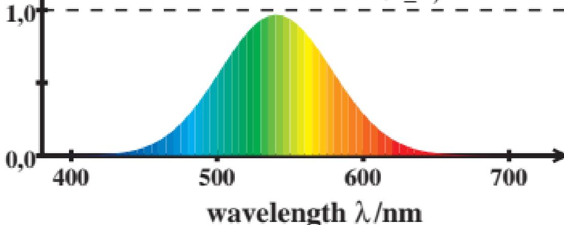
LMS\_F02\_L cone sensitivity  $\bar{y}_{\max}(\lambda)=1$
