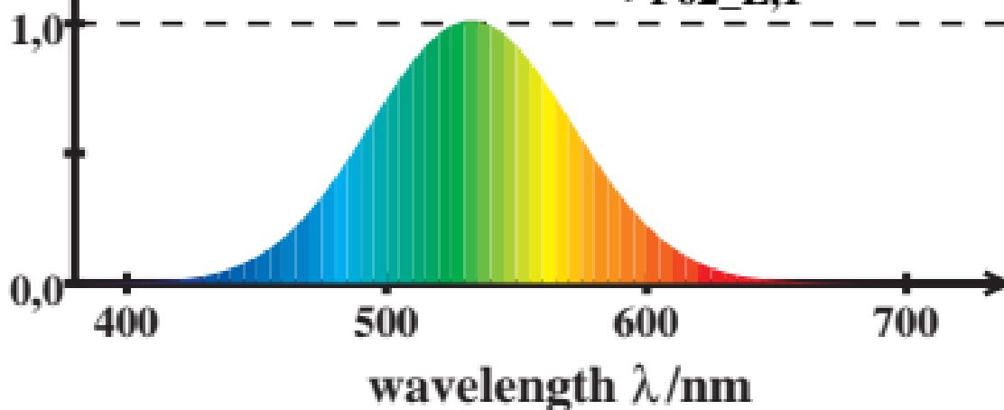
LMS\_F02\_L cone sensitivity  $\bar{y}_{\max}(\lambda)=1$
