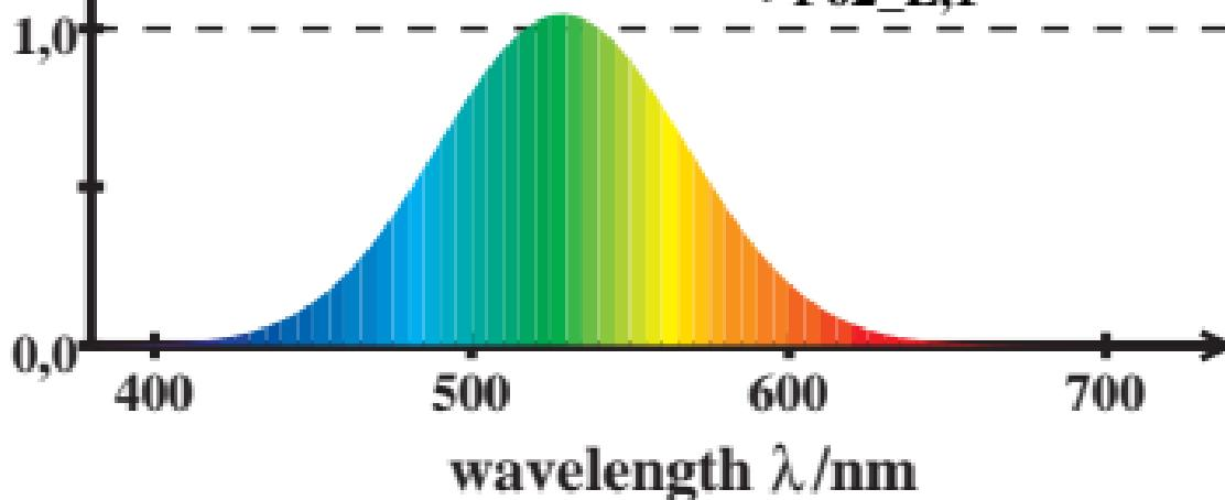
LMS\_F02\_L cone sensitivity  $\bar{y}_{\max}(\lambda)=1$
