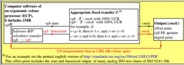
**Colour management by a change of the *rgb* data within the colour workflow before the linearized output**
