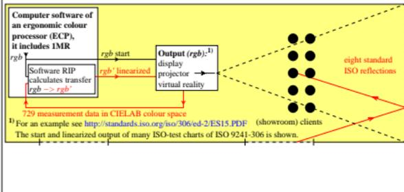
**Colour management by a change of the *rgb* data within the colour workflow before the linearized output**
