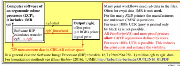
**Colour management by a change of the *rgb* data within the colour workflow before the linearized output**
