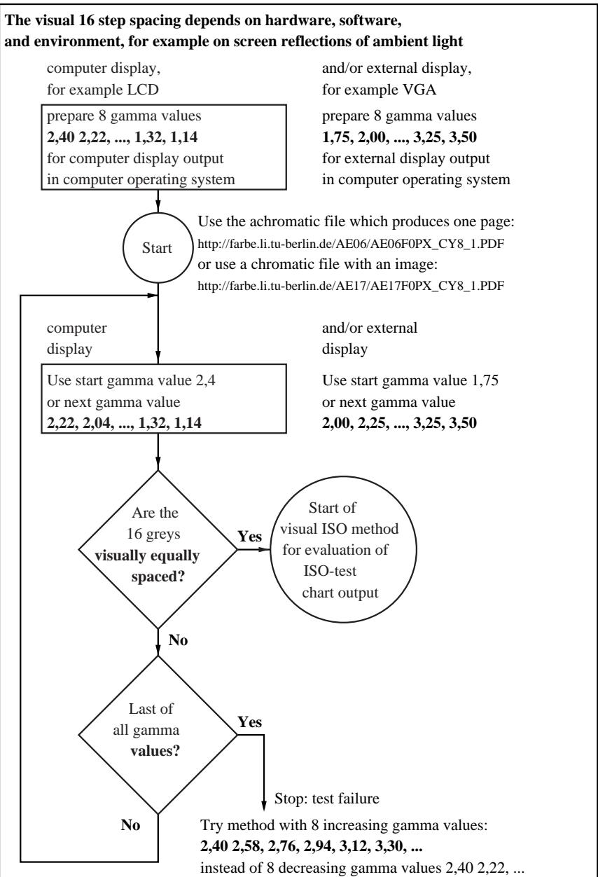
TUB-test chart AE84; Display Output Linearization
