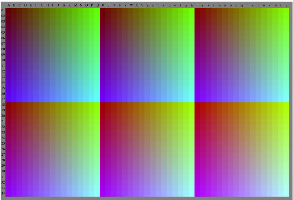
YE380-7N, Test chart with 51x34=1734 separate and adjacent colours; digital 17 step scales; rgb colour data, patch sizes; 4,2mm x 4,2mm and 4,8mm x 4,8mm, Page 1/3
