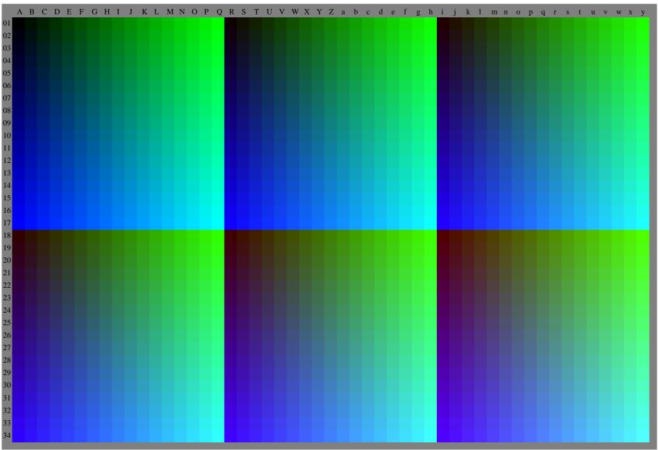
YE370-7N, Test chart with 51x34=1734 separate and adjacent colours; digital 17 step scales; rgb colour data, patch sizes; 4,2mm x 4,2mm and 4,8mm x 4,8mm, Page 1/3
