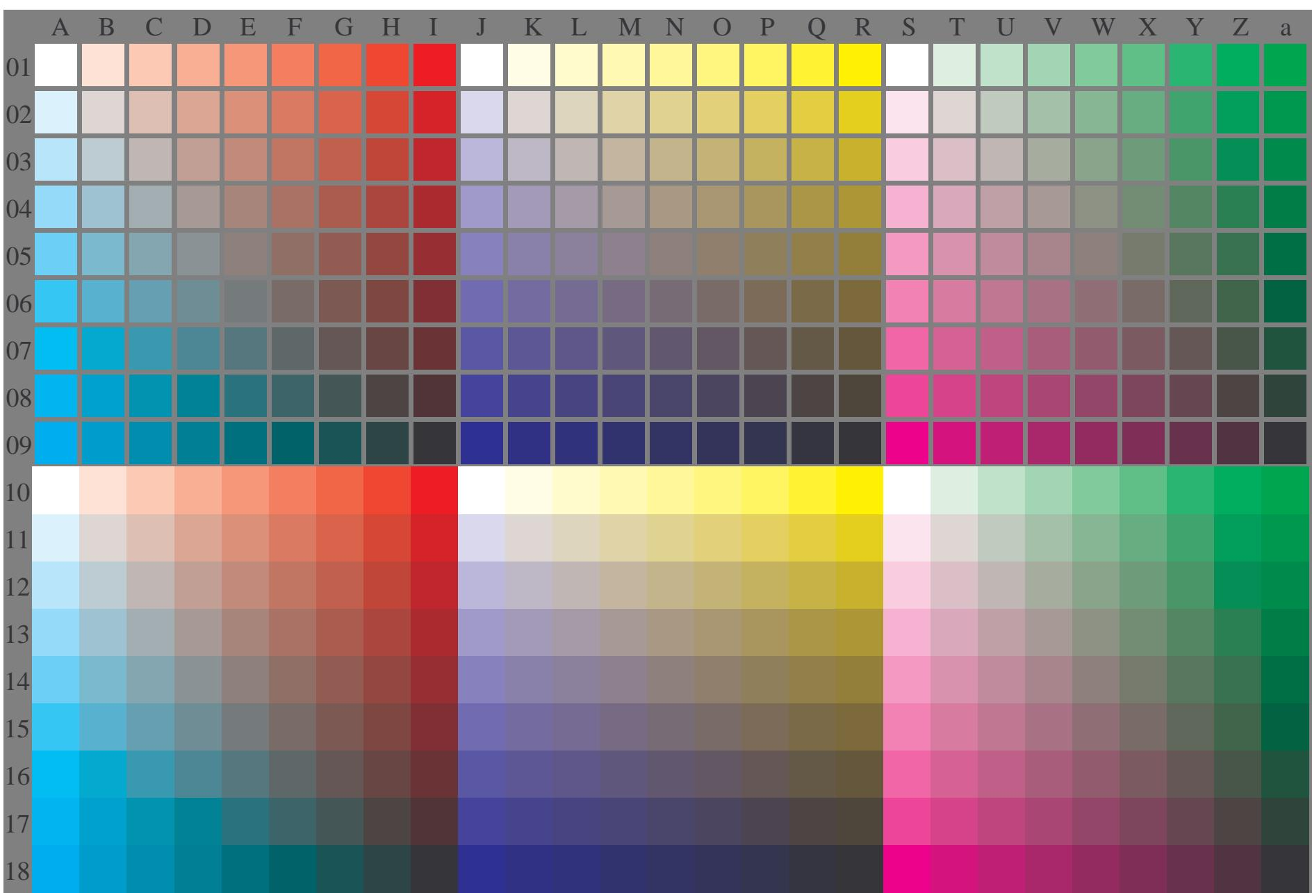
YE340-7N, Test chart with 27x18=486 separate and adjacent colours; digital 9 step scales; compare ISO/IEC 15775; cmy0 colour data, patch sizes: 8mm x 8mm and 9mm x 9mm, Page 1/3
