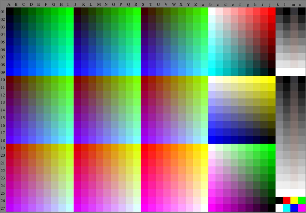
YE240-7N, Test chart with 40x27=1080 colours and digital equidistant 9 step colour scales; compare ISO/IEC 15775; rgb colour data, patch size and grey layout: 6.0mm x 6.0mm, 250mm x 170mm, Page 1/3
