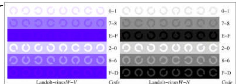
With Linearization: The Landolt-rings are recognized.
