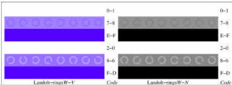
Without Linearization: The Landolt-rings are not recognized.
