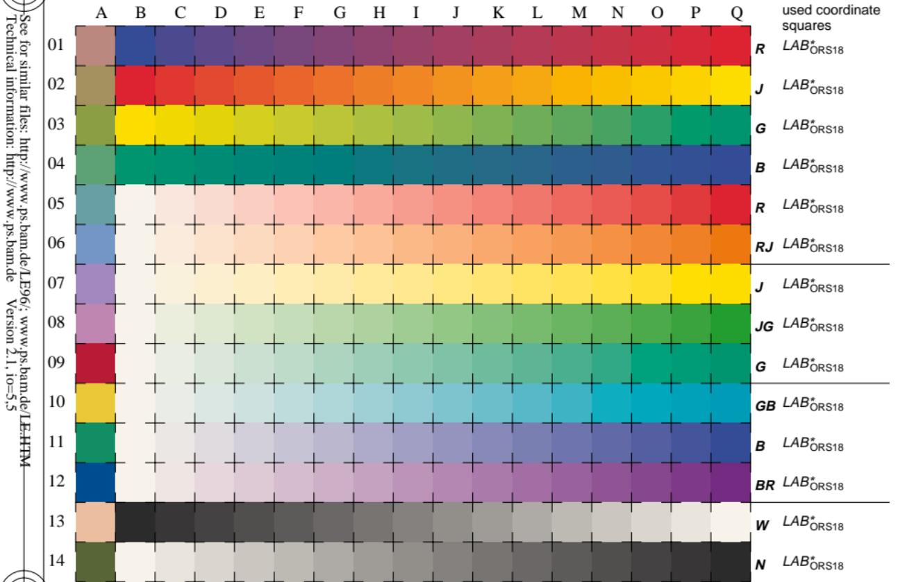
LE960-7, 16 equidistant CIELAB steps in cmy0% (ORS18) for colour series B-R, R-J, J-G, G-B, W-R, W-RJ, W-J, W-JG, W-G, W-GB, W-B, W-BR, W-R, W-N, N-W and 14 CIE-test colours (left)
