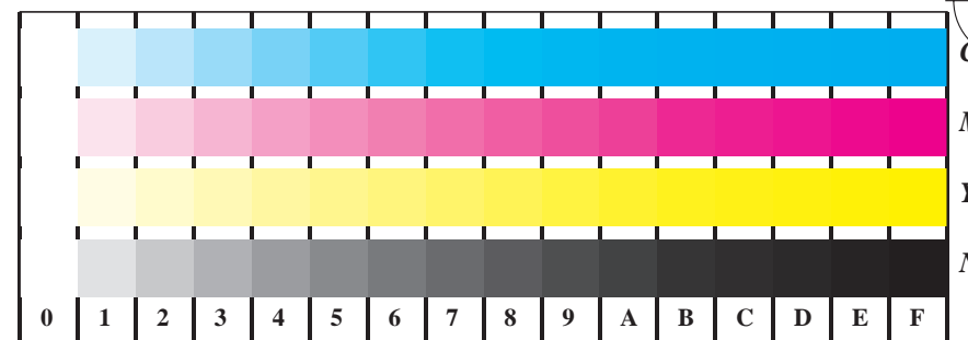
Picture B4w: 16 equidistant steps W-C , W-M , W-Y and W-N ; PS operator cmy0^* setcmykcolor (only)
