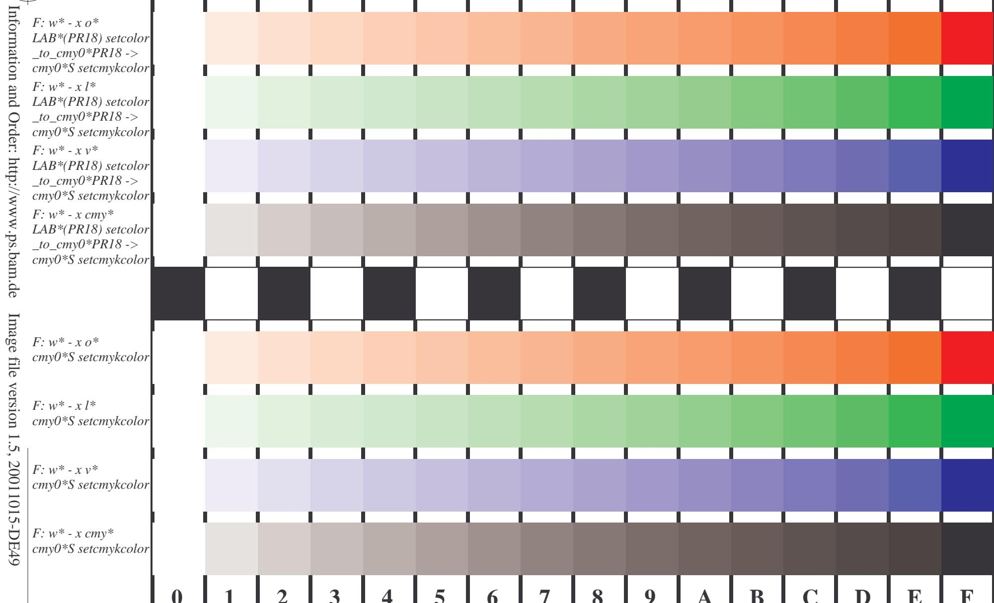
Figure B4 and/or D4 of the ISO/IEC-test charts;  $w^* - cmyn^*$ ;  $w^* - olv(cmy)^*$ ; 16 visual equidistant steps of colour series:  $LAB^* \rightarrow \Delta LAB^*$ ; LM methods: N, F, S, D, T, E
