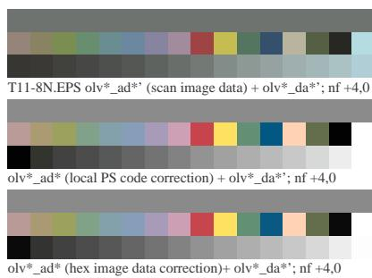
Test chart no. 3700 for input and output (IL, OL): Input Hex data correction by inverse setcolortransfer
