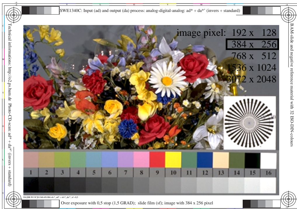
Figure 3: Fig. B1 of test chart according to ISO/IEC 15775 for slide film (0.5 stop overexposure)
