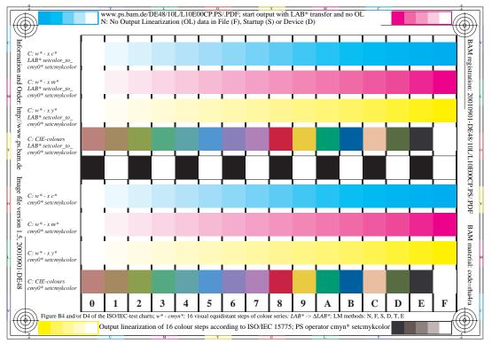
Figure 16: Use of LAB\*\_to\_cmy0\* setcmykcolor and cmy0\* setcmykcolor for the 48 cmy\* standard colours and the 16 CIE-test colours of the ISO/IEC-test chart no. 2.
